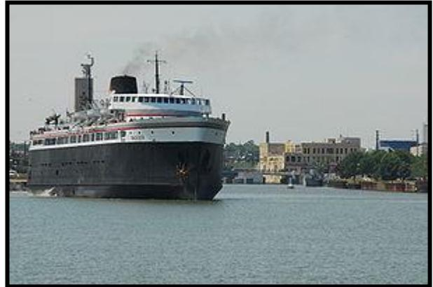
The 410-foot vessel travels between Ludington and Manitowoc. The Badger began hauling rail cars on the lake in 1953 and was refurbished to carry passengers and their vehicles in the early 1990s. It's the nation's last steamship powered by coal.
