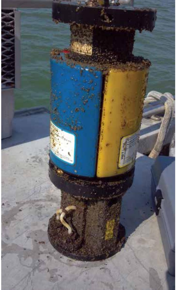
Figure 2. LOBO platform. Float and telemetry are visible; sensors are submerged.
