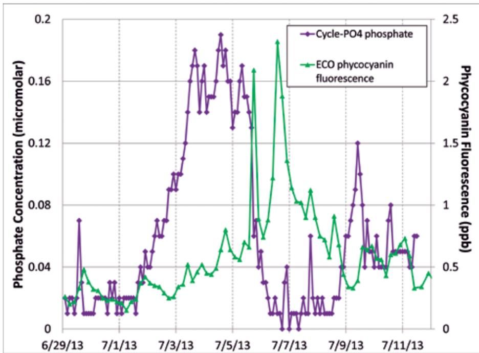
Figure 5. Preliminary, real-time, continuous monitoring data from WLE LOBO. In-situ phosphate concentration is shown in purple, with phycocyanin fluorescence in green. A pulse of phosphate into the system results in a bloom three to four days later, demonstrating the predictive capacity of continuous nutrient monitoring.
