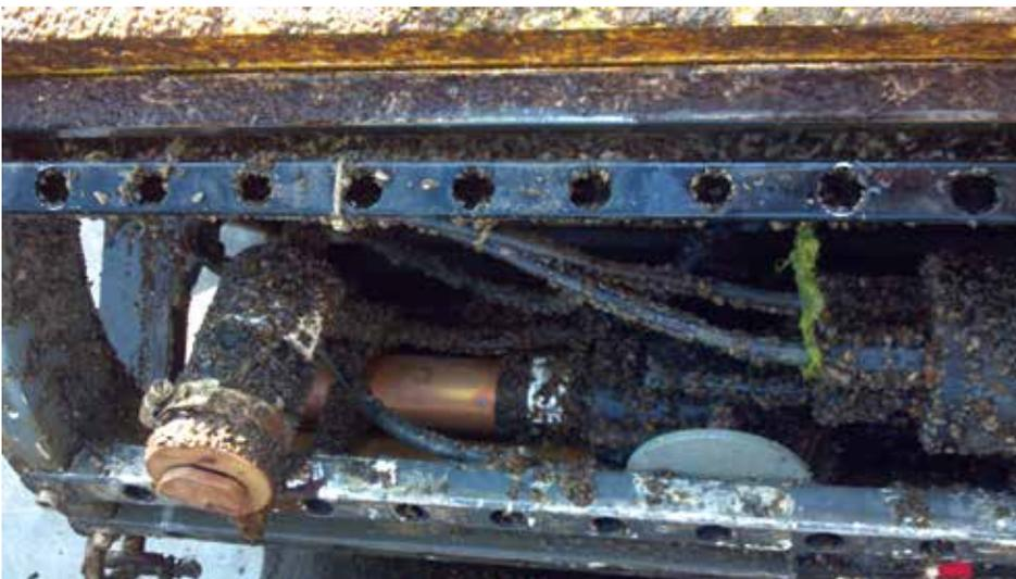
Figure 4. Underside of LOBO buoy, showing bio-optics and CTD. Note that copper surfaces and optical wipers keep measurement surfaces free of fouling.
